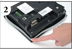
Lay the new gasket over the channel so that the long and short sides of the gasket match up to the long and short sides of the touch panel. Start at one corner and match the gasket's corner to the channel's corner. Press the gasket into the channel and work all away around the perimeter of the touch panel. Re-install the touch panel.
