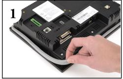
Start at one corner and pull the old gasket out of the channel that holds the gasket in place. Pull the gasket up as you work around the entire perimeter of the touch panel. Discard the old gasket.
